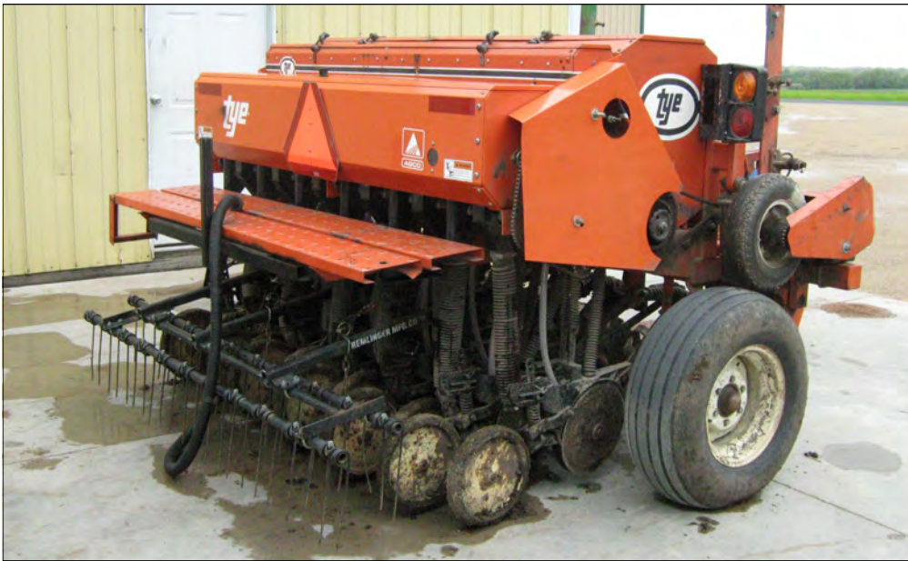
Figure 5. Native seed drills are the ideal tool for large planting sites (5+ acres). Typical models can plant in a light stubble layer, have depth controls for optimal seed placement, and have separate seed boxes for different sizes of seed. Such drills need an experienced operator and careful calibration.
