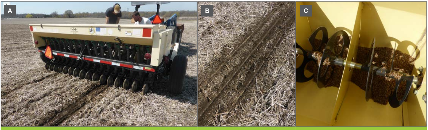
Figure 54—left to right: Most pollinator plantings are established using specialized drills and equipment. These plantings often follow herbicide applications or other season-long site preparation. Typical native seed drill models (A) can plant in light stubble (B), have separate seed boxes for various seed sizes (C), and have depth controls for optimal seed placement. (Photos: Sarah Foltz Jordan, Xerces Society.)
