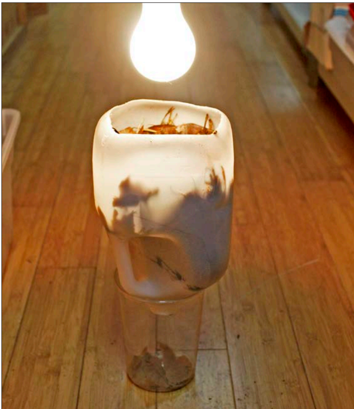
FIGURE 23—A homemade Berlese funnel. The soil sample is held in an upper container that has an open, narrow base (inverted milk jug) on top of a lower container (jar). Over the course of hours and days, heat and light drive the soil invertebrates away from the light bulb source and into the lower container.
