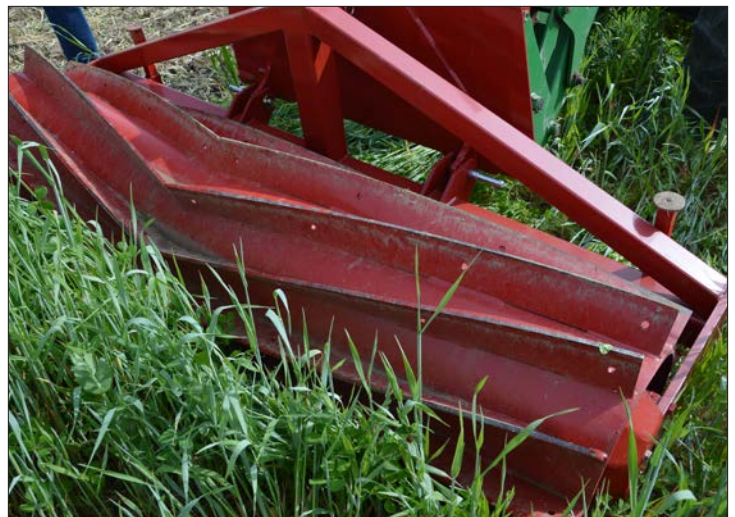
FIGURE 38—A roller crimper is an implement that breaks and flattens the stems of cover crops. This is a non-chemical termination method with minimal soil disturbance.
