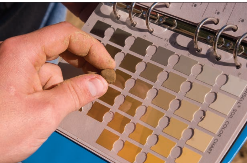
FIGURE 7—A Munsell chart is used to categorize the color of a soil.
