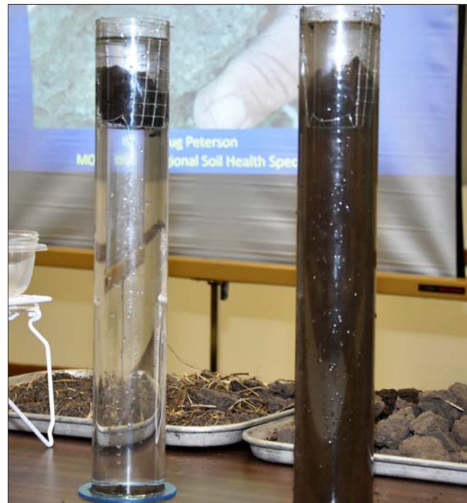
FIGURE 25—In the slake test demonstration, a soil sample with good aggregate stability (left side) remains intact when suspended in water, while a soil sample with poor aggregate stability falls apart.
