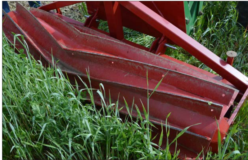
FIGURE 38—A roller crimper is an implement that breaks and flattens the stems of cover crops. This is a non-chemical termination method with minimal soil disturbance.
