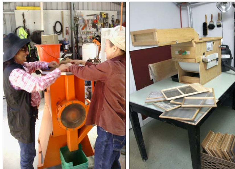
Figure 12: Mechanical thresher (left) 1 and seed cleaner (right) 2 used to clean native wildflower and grass seeds for restoration projects.
